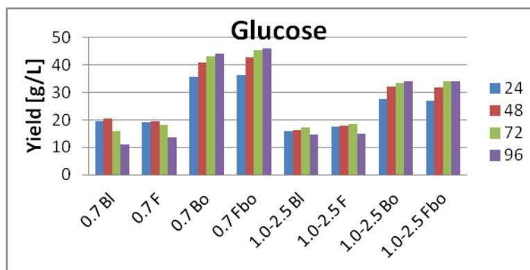
Fig. 2: The yields of glucose of pretreated branch wood beech fractions after enzymatic hydrolyses. Bl = blank; F = deep freezing at  $-80^{\circ}\text{C}$ ; Bo = boiling at  $160^{\circ}\text{C}$ ; Fbo = boiling at  $160^{\circ}\text{C}$  and subsequent deep freezing at  $-80^{\circ}\text{C}$ .
