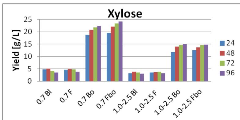
Fig. 3: The yields of xylose of pretreated branch wood beech fractions after enzymatic hydrolyses. Bl = blank; F = deep freezing at  $-80^{\circ}\text{C}$ ; Bo = boiling at  $160^{\circ}\text{C}$ ; Fbo = boiling at  $160^{\circ}\text{C}$  and subsequent deep freezing at  $-80^{\circ}\text{C}$ .
