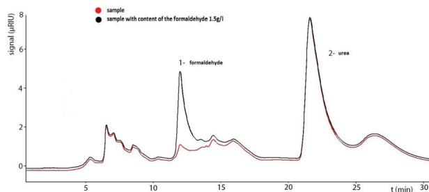
Fig.1: HPLC analysis of the particle board sample by method of internal standard.
