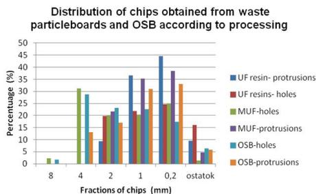
Fig.3: Composition of chips from particleboards and OSB after the cooking treatment and the subsequent disintegration using the mechanism with protrusions.
