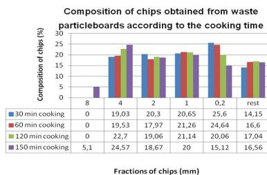
*Fig.2: Fractions of particleboards after the treatment in boiling water and disintegration using the disintegration mechanism with oval elongated holes (5.5 mm x 54.1 mm).*
